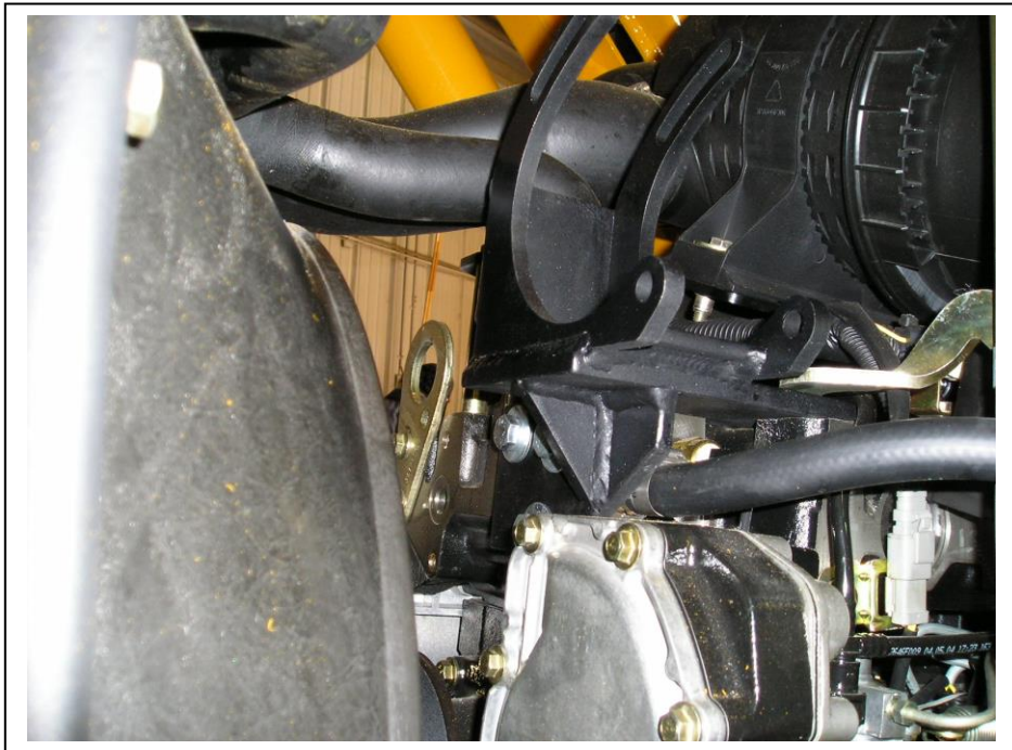
Three M10 x 30mm bolts and large OD flat washers.
